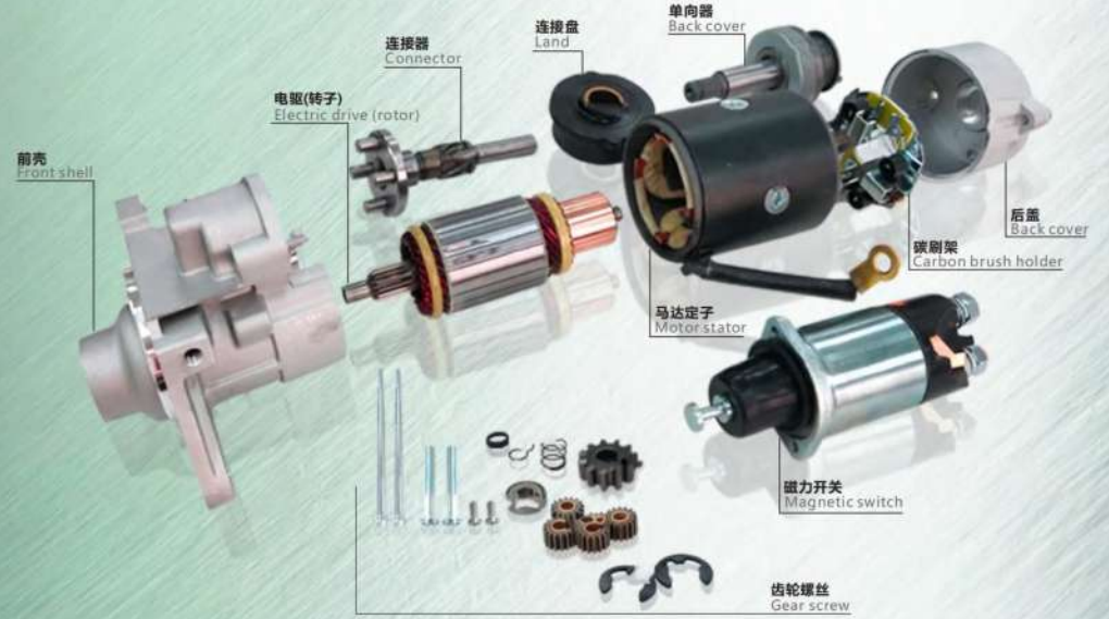
Construction machinery Starter motor exploded view
