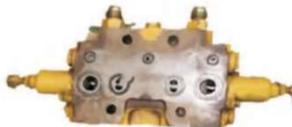
PC120-6(小机头)炮阀 Standby valve hydraulic hammer
