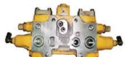
PC-228US-3炮阀 Standby valve hydraulic hammer
