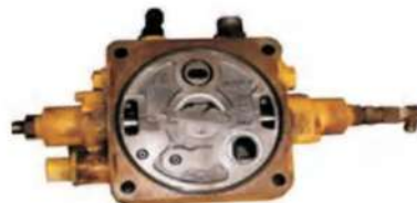
PC120-6(大机头)炮阀 Standby valve hydraulic hammer
